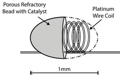
Figure 1: Pellistor Image from City Technology:
