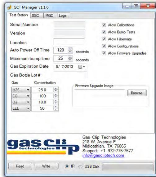
The GCT Manager software can communicate with the Clip Dock through IR or USB as selected by the radio buttons. IR communication is handled through Bay 1 of the Clip Dock and if the IR Link is placed into Bay 1. For IR communication, connect the Clip Dock to a charger and place the GCT IR Link into Bay 1. Direct USB operation with the memory stick connected to the PC offers faster transfers or configuration without a GCT IR Link.
