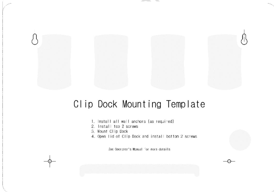
2. Screw the drywall anchors into the marked locations.
